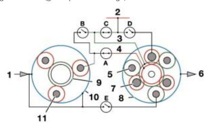
**Power Flow in 3rd Gear:** As in 1st and 2nd gear, drive clutch A is engaged. Drive clutch B is now also engaged. Both sun gears in the double planetary gear train are driven (reaction). As a result, the gear train moves as an assembly and the gear ratio is achieved only by the front single planetary gear train (gear up - ratio change).
